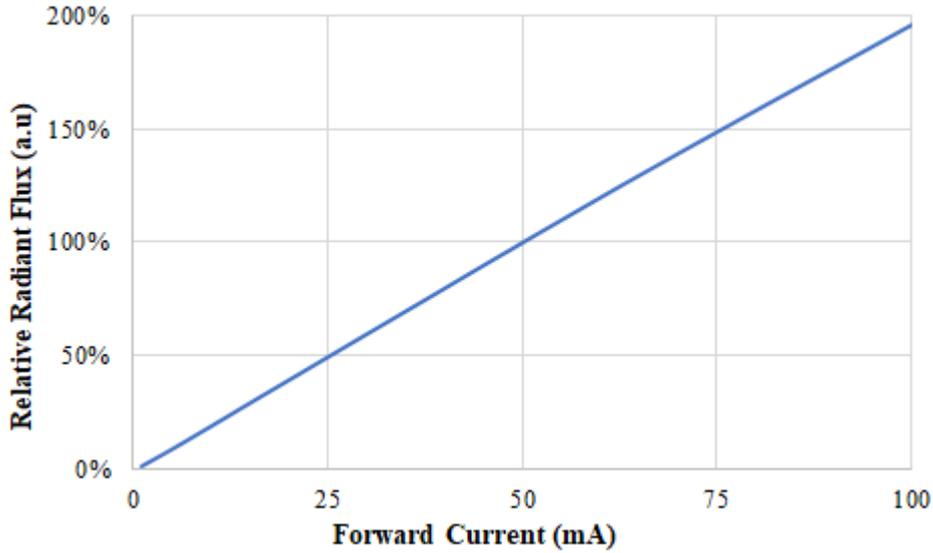
Fig 1. Relative Radiant Flux vs. Forward Current
