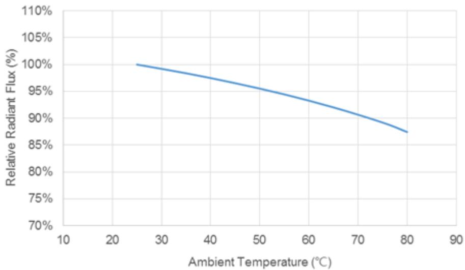
Fig.4 Relative Radiant Flux vs Ambient Temperature
